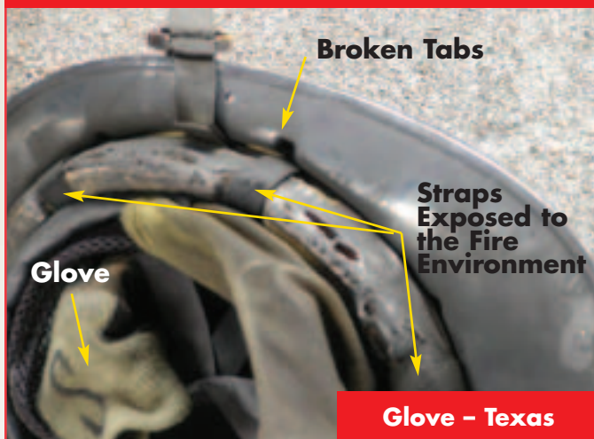
Photo 5 – Broken Tabs – Texas
