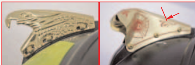
Morning Pride – After One Waist-high Drop Competitor "C" – After ONE Waist-high Drop
