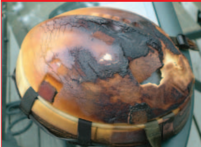
Photo 6 – Expanded/Burnt Foam – Ohio
